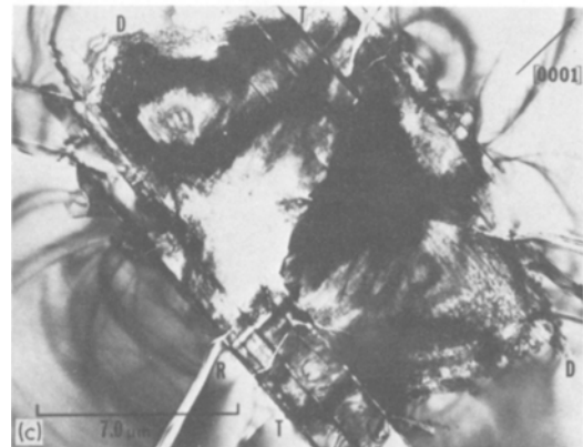
Figure 5 Transmission electron micrographs of Vickers deformation/fracture patterns in (a) Si, (1\ 1\ 2) surface, at 1.00\ \text{N} , (b) SiC (0\ 0\ 0\ 1) at 2.00\ \text{N} , (c) \text{Al}_2\text{O}_3 (1\ 1\ \bar{2}\ 0) at 2.00\ \text{N} , room temperature specimens. Note deformation elements D (dislocations) and T (twins), fracture elements L (lateral cracks) and R (radial cracks). Scale markers in this figure correspond in length to measured deformation zone parameter a (see Fig. 2). (Fig. 5b, after [4].)
